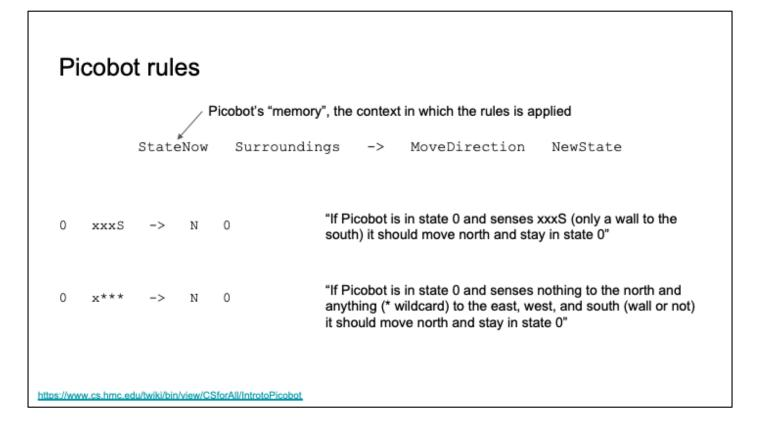
Note that in each step the applicable rules for the current state are checked in order from top to bottom and selects the first rule that applies and then repeats that process in the next step.
