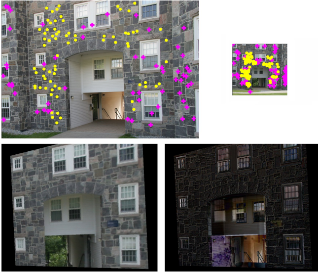
Figure 4. Alignment performance in the presence of significant scale and viewpoint changes. Top row: Cropped regions of a matched image pair. Yellow dots mark features belonging to the model; magenta crosses mark other features. Bottom left: The second image warped by the aligning homography. Bottom right: The difference image visualizing the quality of the alignment (dark regions indicate low differences). Note that the building wall is perfectly aligned.
