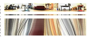
Fig. 1. A sample panoramic view from the robot's omnidirectional camera, the circular 1D image formed by averaging the center scanlines of the panoramic view, and the epipolar plane image (EPI), a "stack" of one-dimensional images over time as the robot travels.
